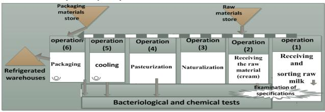
Figure 3. The production process path in the cream Factory
